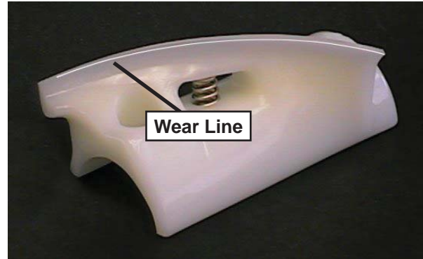
Figure 3-3 Auger Flight Wear
